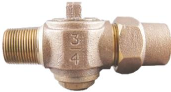
The corporation stop is considered the initial control valve of the service line as it allows for the installation of a new water service line without interrupting the water main pressure. As a special stop valve that is installed into the water main, the corporation stop is usually used only once. However, it may be utilized again in the instance that water needs to be shut off deep below the ground for one reason or another.
